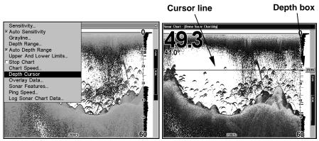
Sonar Page menu with Depth Cursor command selected (left). Sonar chart with the depth cursor active (right). The line indicates the large fish is 21.95 feet deep.
